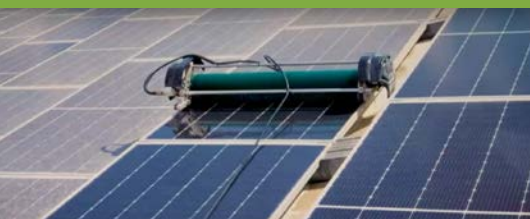
Co-bots are used to clean the panels a minimum of monthly to ensure optimum functionality.
